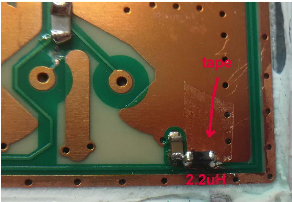
The 2,2 uH inductor must be soldered to the capacitor and to the thin track leading to the F-connector. Use some adhesive tape under the inductor to avoid a shortcut with the large copper area. Positioning of the inductor is critical, because the space in the enclosure is very limited.
